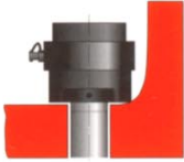
Insufficient flat area around the bolt
