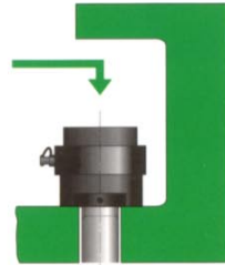
Design enough clearance to install the tensioner
