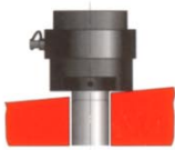
Bearing area is slanted with respect to the bolt axis
