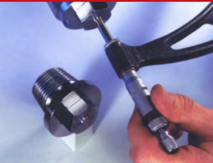
**Pilgrim's Datum Plug provides a simple aid in measuring the length of the Hydraulic Radial Fit Bolt.**
