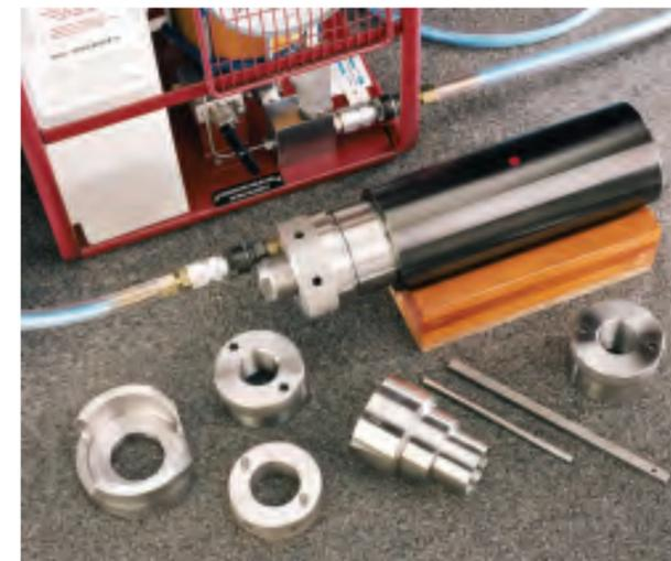
**The training kit is lightweight, safe and easy to handle and can be used in either a workshop or training facility without the need to access the turbine itself.**
